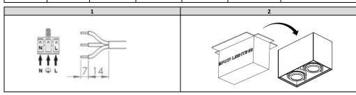
The light source of this luminaire is not replaceable Installation kit supplied with the luminaire does not include anchors for installation.
