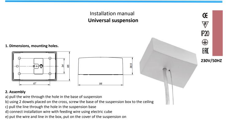
a') in the simple suspension screw the base of the suspension to the ceiling pull the line through the nut, screw it into the base of suspension
